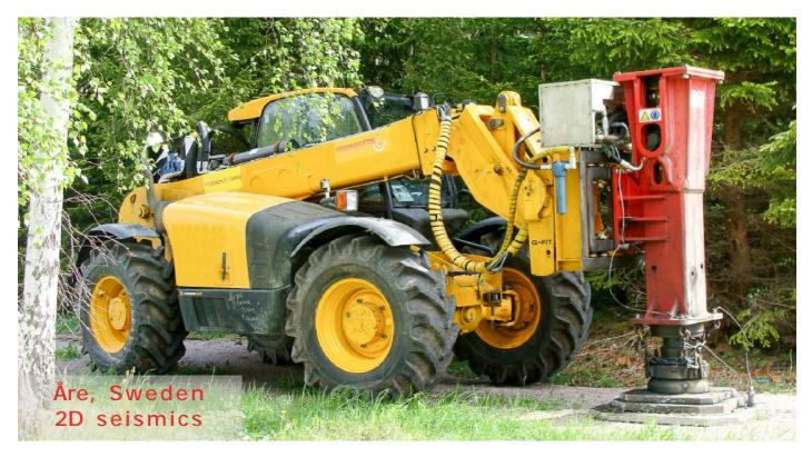
The hammer is powered through a computer controlled hydraulic regulator and produces series of impacts, delivered according to pre-programmed time functions. The recommended temperature range for operation is -30° to 50°C.
