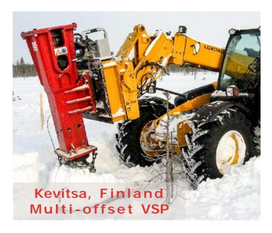
The VIBSIST-3000 produces wide-band seismic signals even when coupling to the ground is relatively poor.
