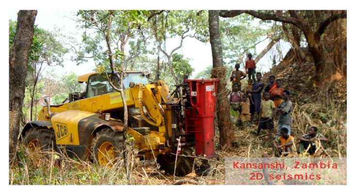
The VIBSIST-3000 uses heavy-duty carrier vehicles and hammers. This makes it safe, reliable and cost effective in difficult terrain as well as in environment sensitive areas, such as forests, rural areas and cities.
