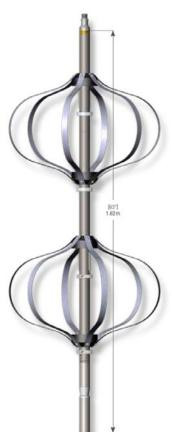
The QL40ABI-VLB (Very Large Borehole) acoustic televiewer is specially designed to assess the integrity of large diameter wells. The tool is implementing the latest hardware/firmware generation to perform casing thickness measurement, corrosion evaluation and cement bond mapping in one run. The tool benefits from new 2G telemetry protocol optimizing logging speed on long single or multi-conductor wirelines.
