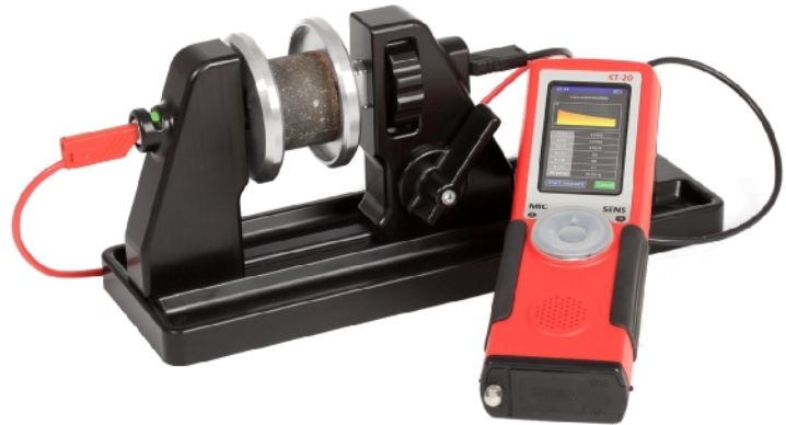
KT-20 Console with IP/Resistivity Sensor (includes Tx-Rx Electronics) and Small Sample Holder
