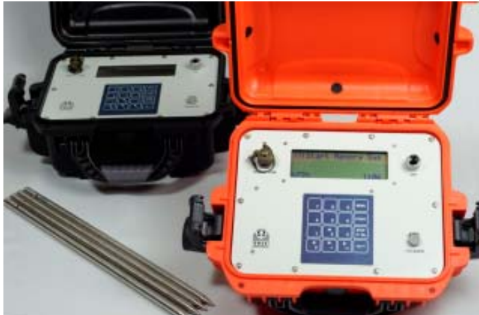
I-Full Waver , compact recorder for full wave signal
