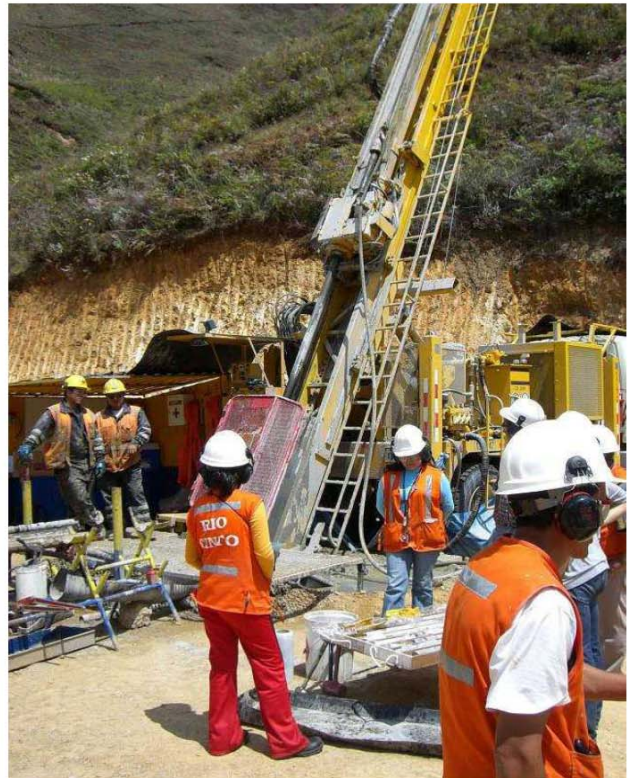
Core extraction at drill site
