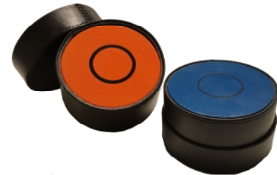
Low and High Range (left and right) Flat Magnetic Susceptibility Calibration Pads
