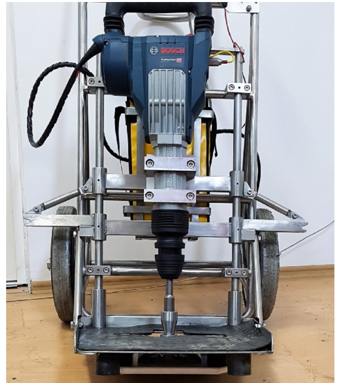
The VIBSIST-50S with Hand Cart and Impact Plate for soft ground.
