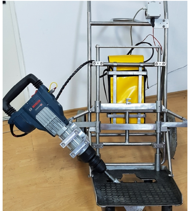
The VIBSIST-50S with Hand Cart and Impact Rod
