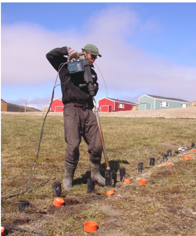
The VIBSIST-20 used in boreholes for tomographic imaging to assess the seismic properties of permafrost in northern Quebec, Canada. Both P- and S-waves are generated
