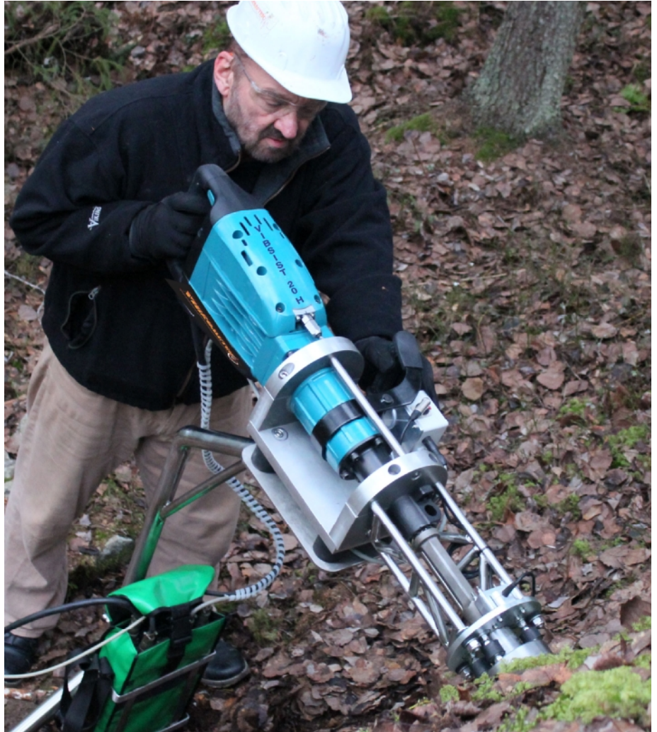
The VIBSIST-50H with Impact Rod and impact head for hard rock coupling.
