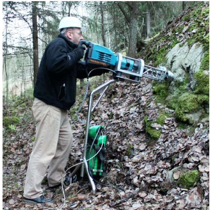
The VIBSIST-20 H used on a vertical rock surface for tomographic imaging to assess the integrity and stability of a steep outcrop.
