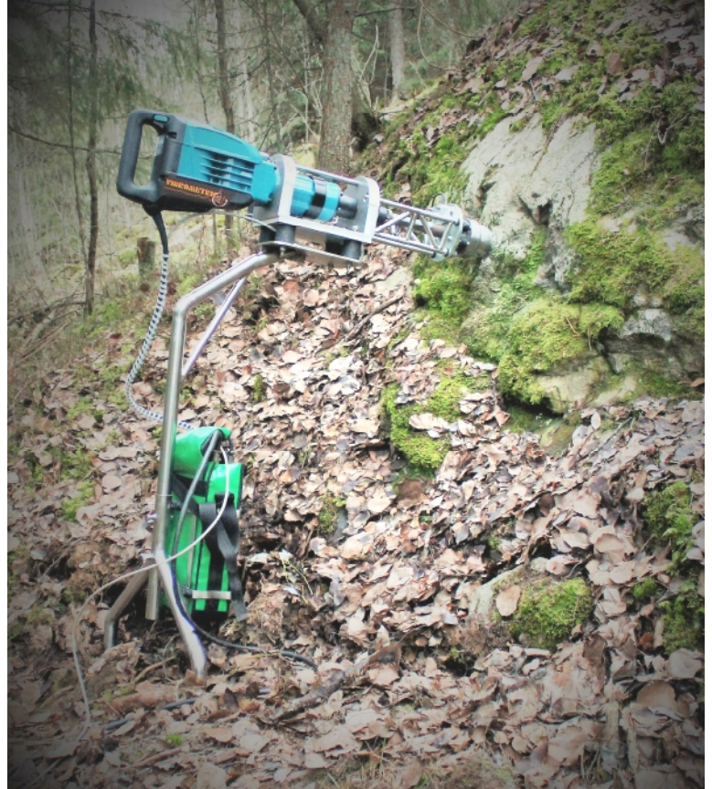
The VIBSIST-50H with Hand Cart and Impact Rod and Coupling Plate for P-S waves.
