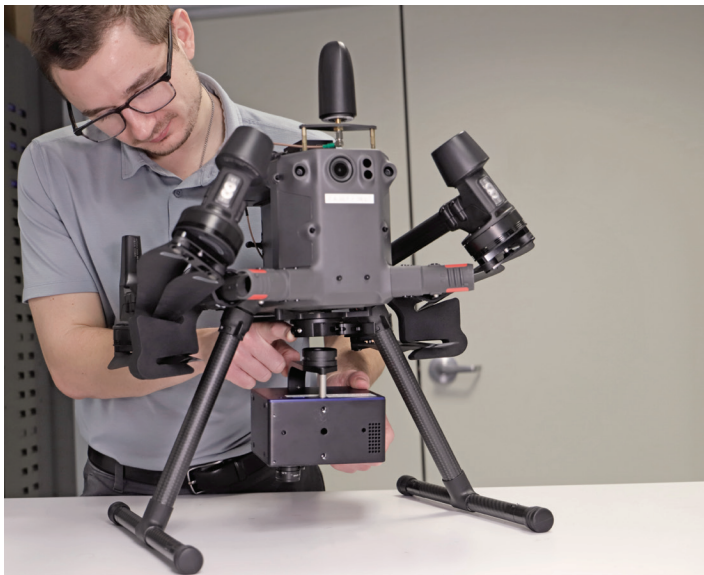
Figure 1. UAV systems utilize a quick-release mechanism between the drone platform and the payload that allows easy removal of the sensor suite for transportation or storage. Some systems may be configured for use on a Field Rotary Kit to gather ground-truth data in the field.
