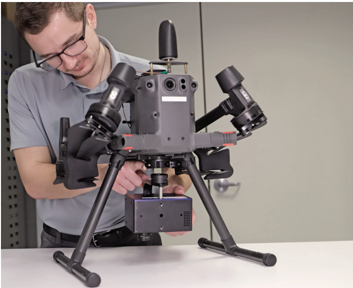
Figure 1. UAV systems utilize a quick-release mechanism between the drone and the payload that allows easy removal of the sensor suite for transportation or storage.
