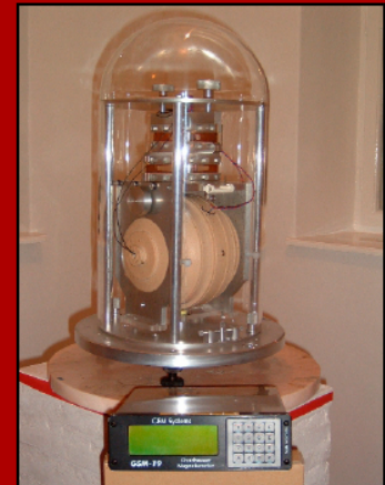
High Precision suspended coil (didd) VECTOR Magnetometer for evaluation of the x, y, z components of the field and monitoring changes in the Declination & Inclination.
