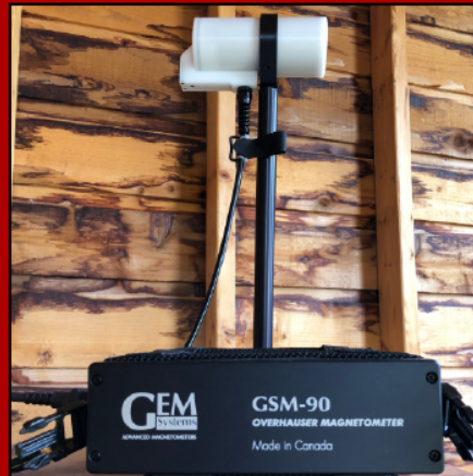
Continuous reading SCALAR Total Field magnetometer for calibration - GEM Systems Robust Overhauser (GSM-90).
