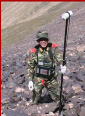
GEM GSM-19T Proton Precession system. The image shows a staff-mounted configuration with console, sensor, supporting pole and cables. A backpack-mounted version, and optional GPS are available for hands free operation.
