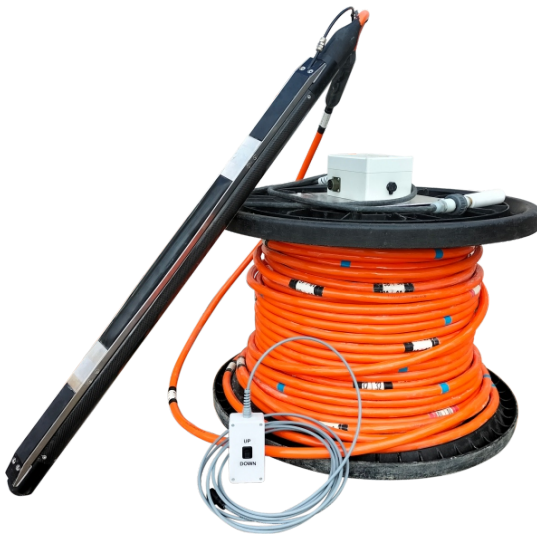
S-wave source BIS-SV on drum and switch box.
