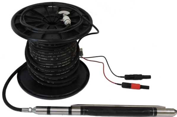
S-wave source BIS-SH-DS on drum with clamping mechanism (inflatable bladder) and connector to the impulse generator IPG800.
