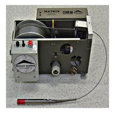
The two mini winches are set at the factory to operate at either 110VAC or 220VAC and cannot run at the other voltage. If the winch is configured for 220 AC, there will be a red label below the POWER IN connector indicating 220 VAC. The Matrix is auto switching between 110 and 240 VAC.
