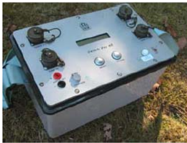
Extension Switch Pro box able to drive 24 - 48 - 72 or 96 electrodes
