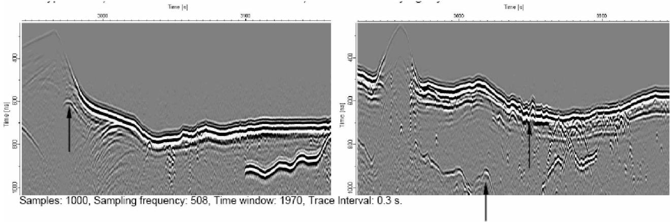
In this example the RTC was used to map a thin soil layer on top of the bedrock (bedrock level marked with green line below), and as a result also larger fracture zone with in the bedrock could also be mapped, represented by the two red lines below.
