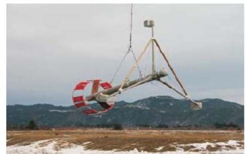
measurements. Here, four Potassium units can be installed in a special “bird” with 2 fins at the tips of an imaginary tetrahedron to allow for measurement of Total Magnetic Field and the gradients in 3 directions:
