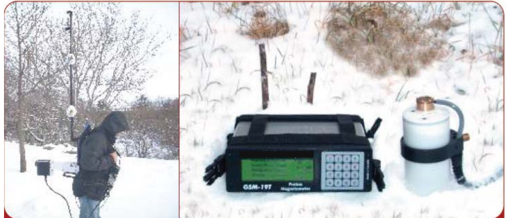
GSM-19T Proton Precession console configured with backpack, additional sensor for gradiometer (simultaneous) readings, built-in GPS and VLF EM system
