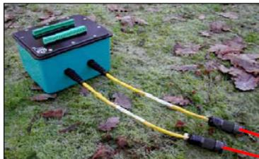
48 terminations strip box for Elrec Pro Switch-48 unit
