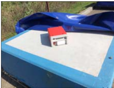
D230A Being Calibrated on Reference Pad
