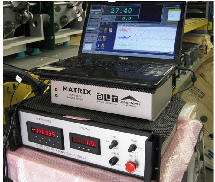
Winch Controller with Matrix Logger Console and Laptop
