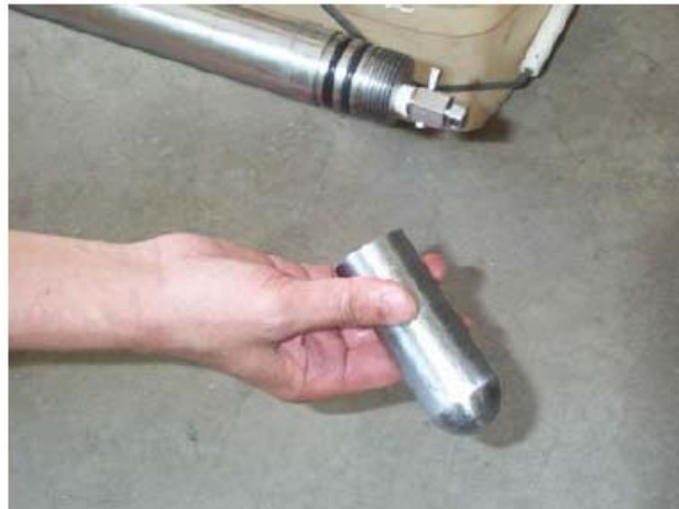
Removing the 1 –liter fluid sample through valve
