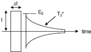
Figure 6. Envelops of the excitation pulse and of the magnetic resonance relaxation signal:  $I$  is the intensity of the current,  $\Delta t$  its duration,  $E_0$  the initial amplitude of the signal,  $T_2^*$  its time constant
