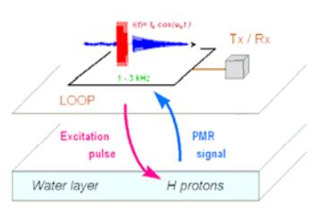
Figure 5: Principle of the magnetic resonance method
